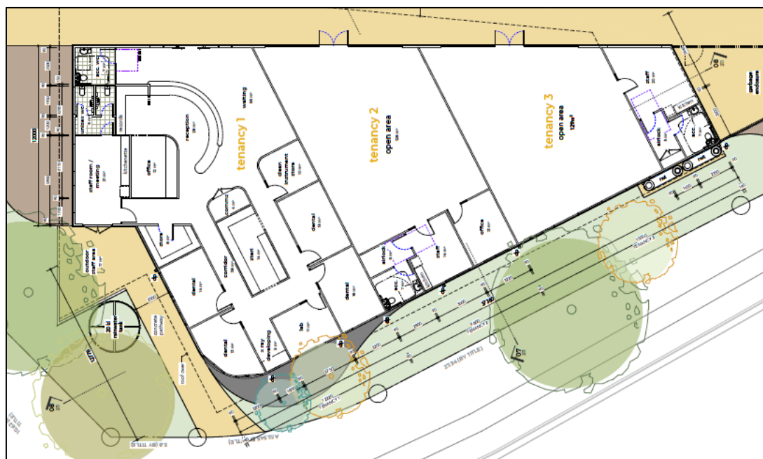
Figure 6: Allied health centre proposed floor plan (source: Barson).
